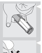
9 Pry the 2 AA-sized cylindrical nickel-cadmium batteries loose by inserting the screwdriver on the sides of the two batteries in the locations shown in the figure.
